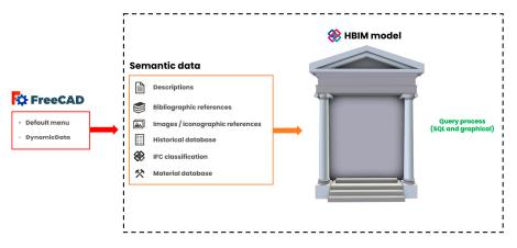
**Figure 8.** Semantic data inclusion is essential for query processes. Default menu and DynamicData WB allow to enrich the parametric model with technical and historical information.
