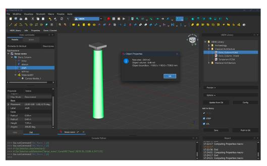
**Figure 5.** HBIM\_Library macro inside FreeCAD for evocating predefined custom parametric models. The column is composed of PART elements such as torus, cubes and cones. The macro is included inside the HBIM workbench.
