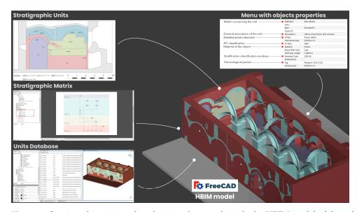
**Figure 9.** Stratigraphic units and analysis implemented inside the HBIM model of the refectory: stratigraphy and interpretation as parametric objects, database, semantic data and images.
