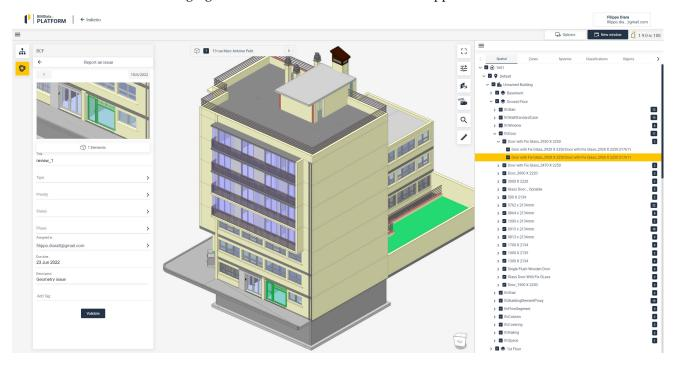
**Figure 10.** BIMData platform: detail of the sample model inside the 3D viewer. On the right side the properties tree; on the left the BCF plugin for generating reviews.
