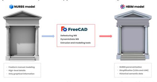
**Figure 7.** From NURBS to HBIM model via FreeCAD open source software: default tools and implemented workbenches for converting NURBS into parametric and informative objects.
