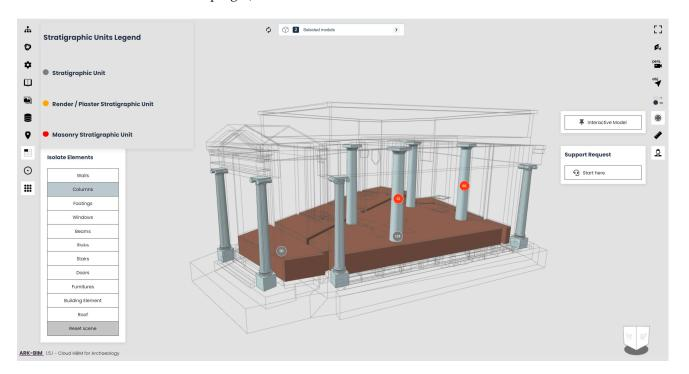
**Figure 12.** The Domus Regia HBIM model inside the ARK-BIM environment. Additional plugins are on the left and right side of the window: details on picked stratigraphic units and "IfcColumn" isolated in the 3D environment.
