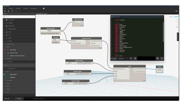
and VPLs have recently started and DynFreeCAD [23] has been composed for integrating the functionalities of Dynamo [24] to FreeCAD software via Python (Figure 4).
