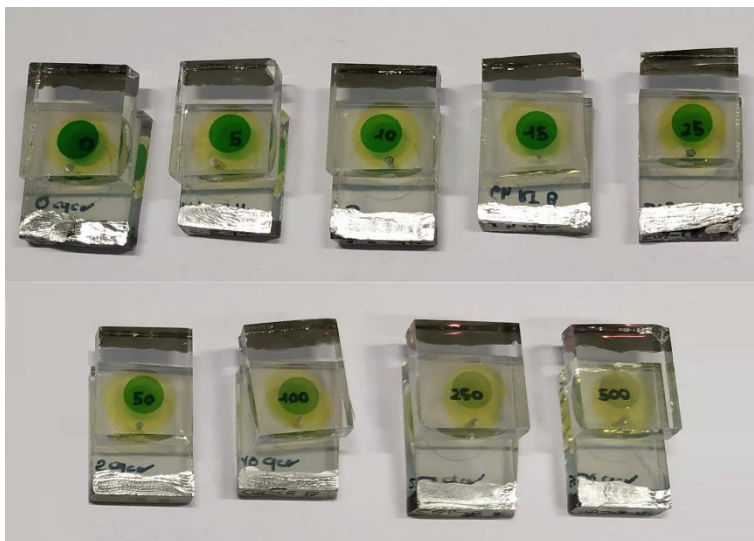
Figure 85 – Photography of DSSCs based on sensitizer 348 obtained using different concentrations of CDCA in the dye-loading solution. The numbers in black are written on the paper below the devices, demonstrating their transparency.
