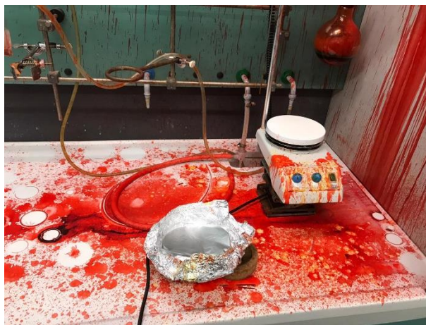
Figure 59 – Uncontrollable outflow of 7 g scale tri-bromination reaction.
