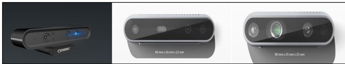
Figure 18: The alternatives to Microsoft Kinect: Astra Pro (left), D415 (centre), D435 (right) [Image source: manufacturer web pages]
