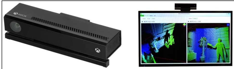
Figure 17: The Microsoft Kinect v.2 (left) and 3D reconstruction of the scene (right) [Image source: https://developer.microsoft.com/en-us/windows/kinect/ ]
