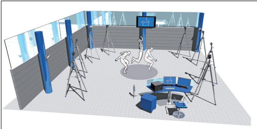
Figure 9: Example of environment dedicated to motion analysis with an optoelectronic system. In this configuration, the system cameras are mounted on tripods and the “grey circular area” represents the working volume in which accuracy of motion capture is guaranteed.
