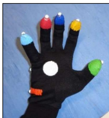
Figure 27: Glove with reflective markers for the optoelectronic system [Image source: Paper 1]
