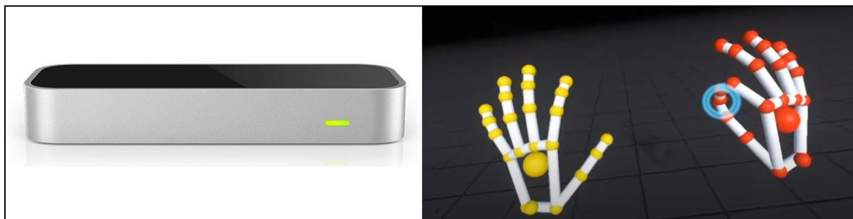
Figure 20: The Leap Motion (left) and the hand skeletal model (right) [Image source: Leap Motion web page]
