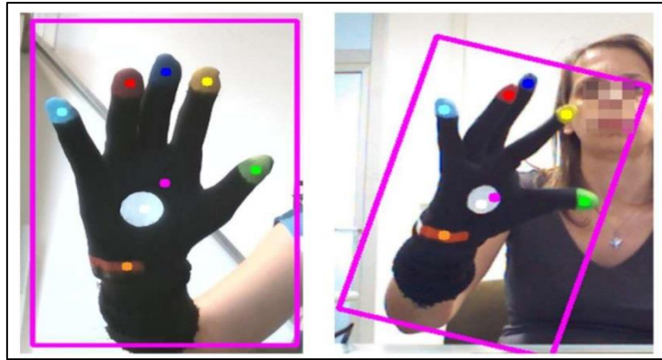
Figure 26: Hand Tracking algorithm: static open hand (left); dynamic semi-closed hand Hand segmentation, detection of color markers, bounding box and centroids of hand with glove and color blobs [Image source: Paper 1]
