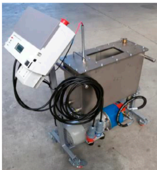
Figure 1. Image of hydraulic test bench realized to age oil.
