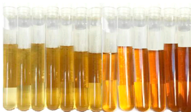
Figure 2. Series of oil samples aged from 0 to 3000 h (step 250 h) through the hydraulic test bench.
