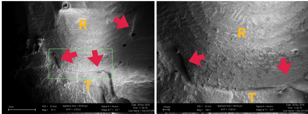
Figure 9. Left picture: SEM image of TRI after thermomechanical loading at 67x magnification. The restoration is marked with “R”, while the tooth with “T”. Specifically, the picture is showing an interproximal area of an indirect adhesive restoration. Right picture: detail (150x magnification) of the green-cornered area highlighted in the left image. It is worth to notice the high quality of the images, that can easily detect defects of the interface, such as cracks and undercuts (red arrows).
