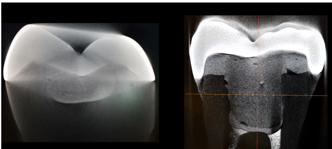
Figure 12. Micro-CT images of the same zirconia restoration, before (left image) and after (right image) optimization. In this case, the point of interest was the cervical and internal area of the restorative material. Thus, sample was positioned properly in order to have artifacts in the occlusal area rather than cervical area. Additionally, 0.5 mm Aluminum and 1 mm Copper filters were applied in the acquisition and a beam-hardening correction was applied in reconstruction (Nrecon, Bruker).
