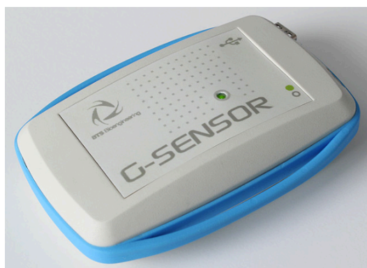
Figure 3 – G-Walk sensor used to evaluate the spatio-temporal parameters of the gait cycle
