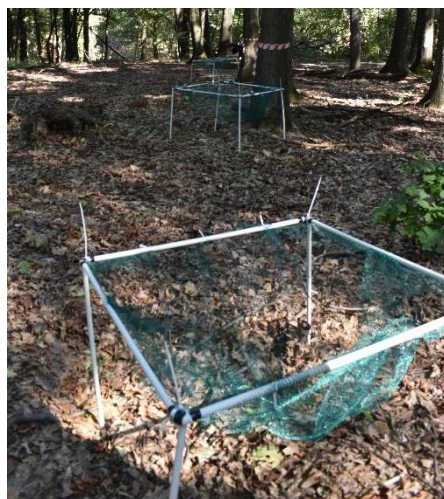
Figure 3.12. Litter traps installed for fresh litter collection at La Mandria Park.
