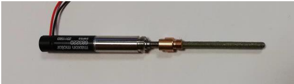
Figure 4: The metal brush motor with the four stages gear reduction system and the preselected screw drive in the assembled configuration.
