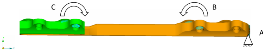
Figure 10: The simplified FE model with constraints and loads applied to this specific plate.
