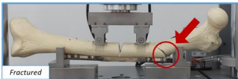
Figure 19: Force-displacement curves obtained from the experimental tests for integer and fractured samples: the red arrow marks the point where the femur broke.
