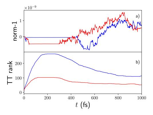
Figure 3: a) Purity of the vibronic model of the pentacene dimer coupled to a bath. Blue line  $\epsilon_{12} = 600 \text{ cm}^{-1}$ ; red line  $\epsilon_{12} = 300 \text{ cm}^{-1}$ ; b) Purity of the vibronic model of the pentacene tetramer coupled to a bath; bath reorganization energy 100 cm<sup>-1</sup>, characteristic frequency  $\omega_c = 50 \text{ cm}^{-1}$ .
