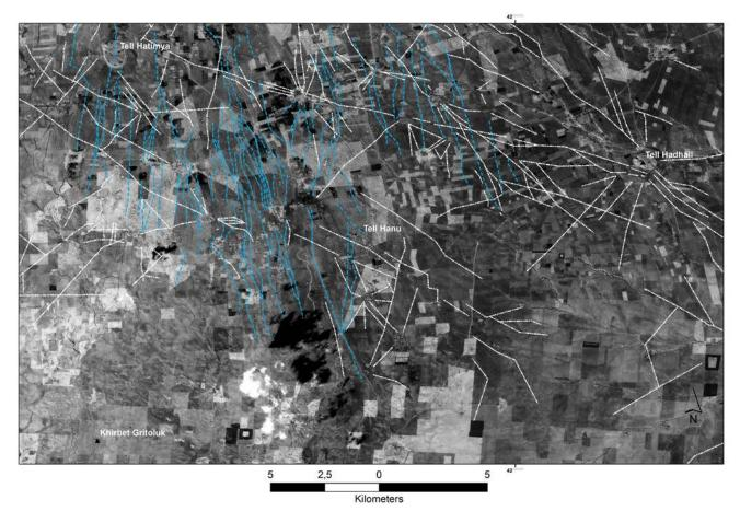
Fig. 11 Area of Tell Hatimya and Tell Hadhail. *Qanats* marked in light blue and hollow-ways in white.
