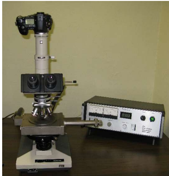
Figure 5.1. The cold-CL apparatus in use at the Earth Science Department of the University of Torino.
