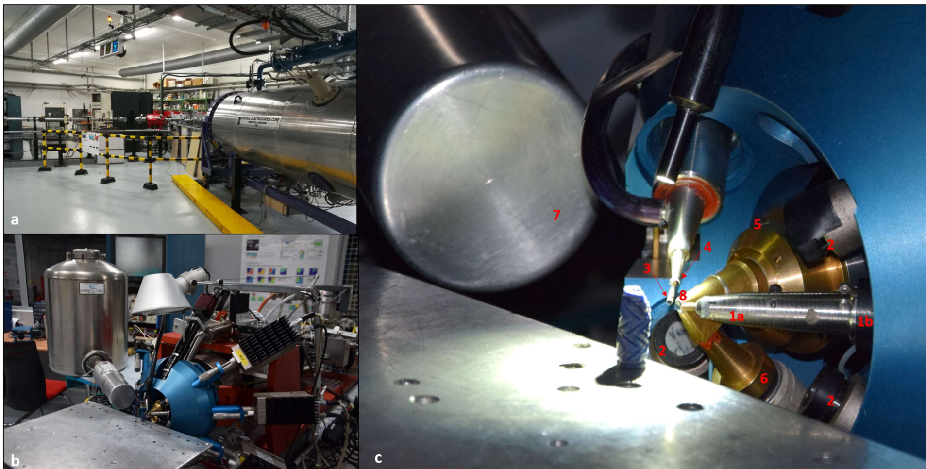
Figure 5.5. NewAGLAE facility. (a) The Pelletron accelerator and the microbeam line; (b) view of the NewAGLAE external beamline setup; (c) zoom on the setup during the measurements on one of our samples. Setup specifics: (1a) He flux magnetic nozzle connected to (1b) low energy SDD detector; (2) three high energy SDD detectors; (3) optical fibre; (4) external RBS detector; (5) annular RBS detector; (6) SDD dose detector; (7) HP-Ge Gamma-rays detector; (8) \text{Si}_3\text{N}_4 exit window.
