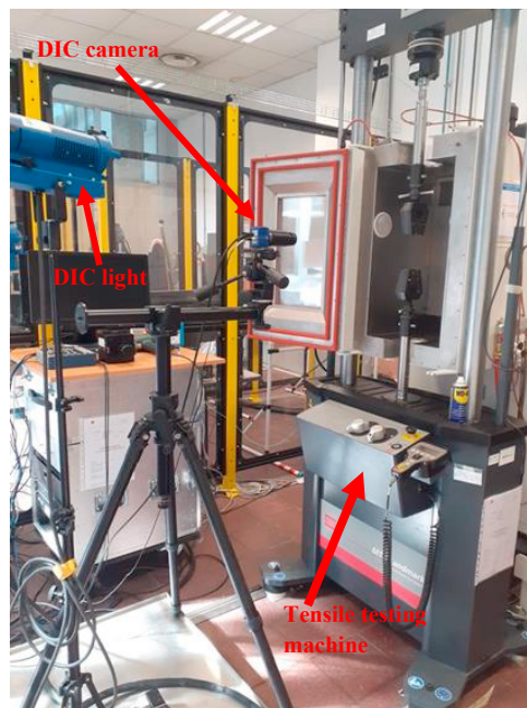
Fig. 4. Tensile testing machine and DIC configuration.
