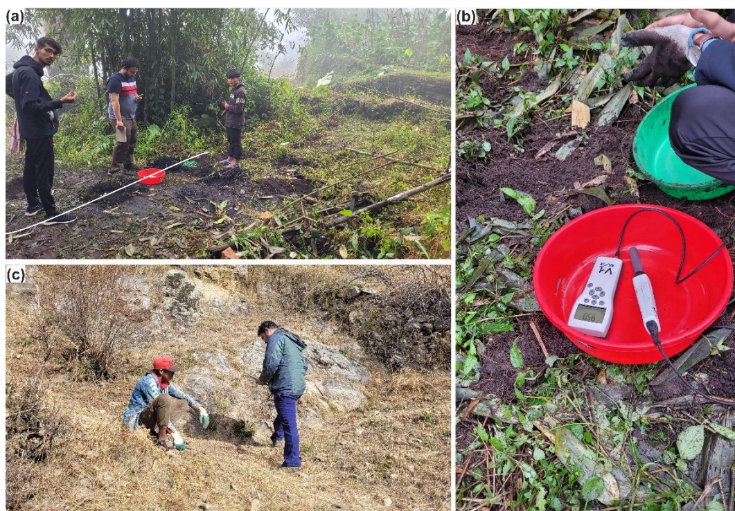
Fig. 3.3: Representative photographs for the measurement of CO 2 gas emission in the field (a) recording the CO 2 flux in the Nundhaki site along the profile shown by the white line in the (b) picture of the CO 2 measuring sensor and the bucket used to cover the sensor. (c) measuring CO 2 from the ground in the Far Western Nepal, Kermi site.
