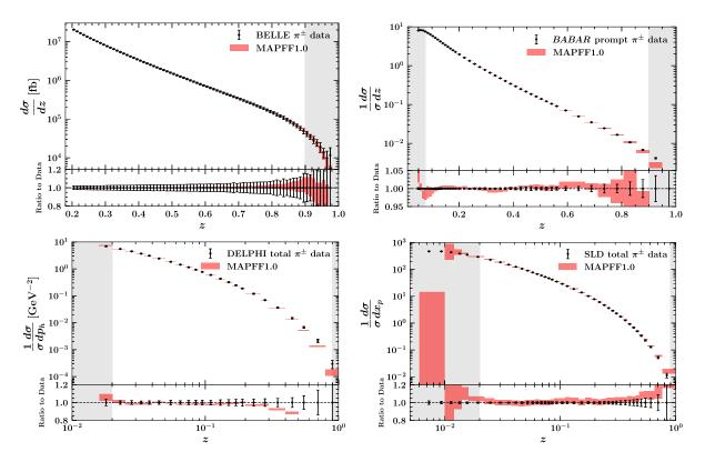
FIG. 2. Top row: data-theory comparison for the *B*-factory experiments BELLE (left) and *BABAR* (right) at  $\sqrt{s} \simeq 10.5$  GeV. Bottom row: representative data-theory comparison for SIA datasets at  $\sqrt{s} = M_Z$  from DELPHI (left) and SLD (right). The shaded regions are excluded from the fit.
