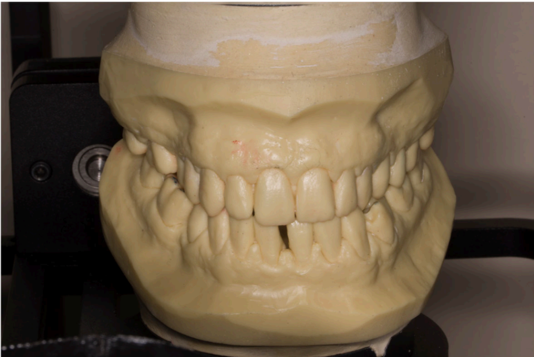
Fig. 9. Models set in the cast holders. Close up image of the upper and lower resin models in the robot cast holders
