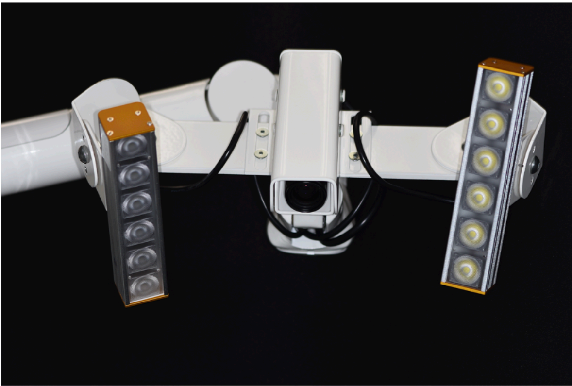
Fig. 4 Bionic Jaw Motion Movement Analyzer. The jaw movement analyzer is composed of a high-speed recording camera and a software running on a computer. The software recognizes the known geometries of the markers and their optical deformation during movement registration thus reconstructing mandibular movement. It is mandatory to check whether the artificial vision software is able to locate reciprocal position of the markers during all opening phases before performing the actual recording.
