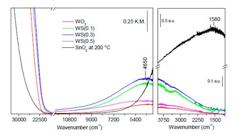
**Figure 3.** FT-IR spectra of W-Sn samples during interaction with  $CO/O_2$  (1:5,  $p_{CO} = 5$  mbar) at the temperature of the maximum absorption intensity.
