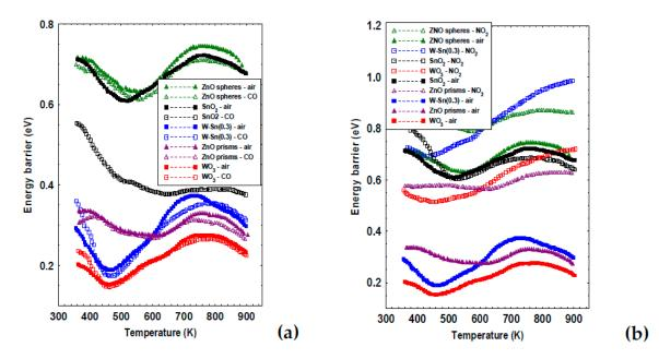
**Figure 4.** (a) Comparison between the energy barriers in dry air and in 100 ppm of CO; (b) in dry air and in 10 ppm of NO<sub>2</sub>.
