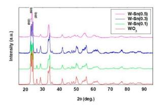
Figure 1. XRD pattern of pure WO<sub>3</sub> and W-Sn powders (nominal Sn molar fraction of 0.1, 0.3 and 0.5).
