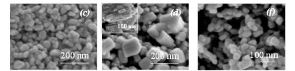
**Figure 2.** FE-SEM images of the calcined powders: (**a**) WO<sub>3</sub>; (**b**) W-Sn(0.1); (**c**) W-Sn(0.3); (**d**) W-Sn(0.5); (**e**) ZnO nanoprisms; (**f**) ZnO nanopheres.
