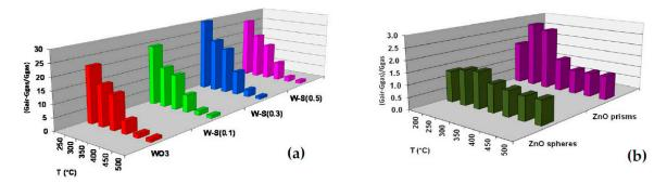
**Figure 5.** (a) Responses of W-Sn sensors to 1 ppm of NO<sub>2</sub> reported as (G<sub>air</sub>-G<sub>gas</sub>)/G<sub>gas</sub> obtained at different working temperatures; (b) responses to 100 ppb of O<sub>3</sub> for ZnO spheres and prisms both fired at 650 °C.
