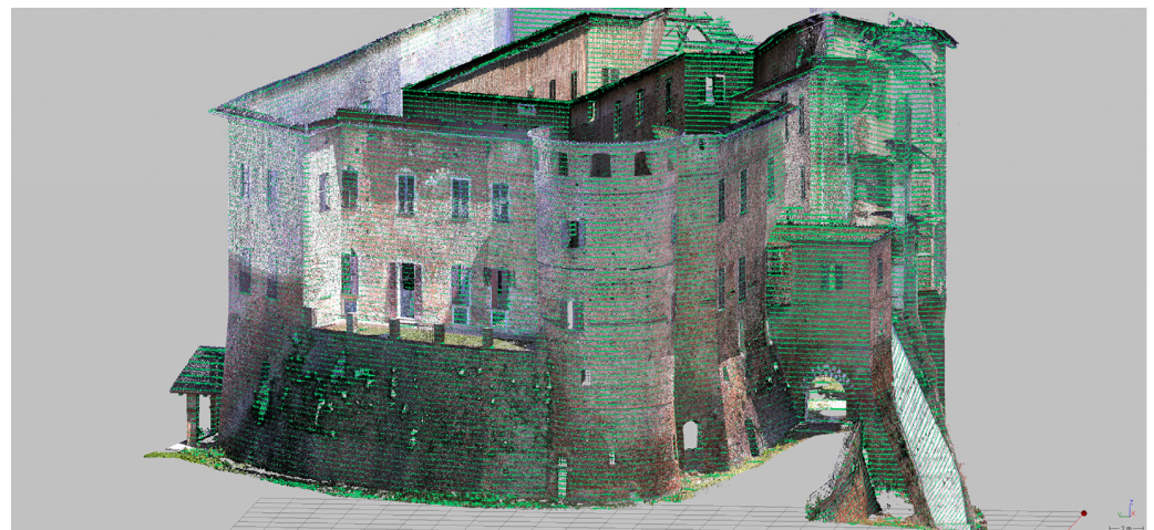
Figure 5. Profiles' extraction from the intersection between the point clouds and planar sections passing through X, Y, and Z planes.
