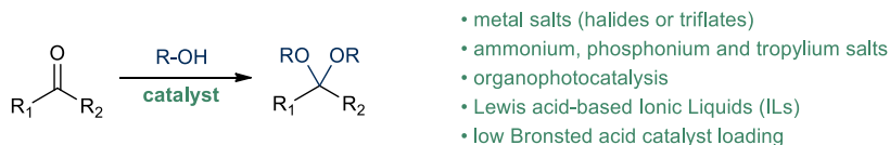
Scheme 3.2. State-of-the-art of the acetalization reaction.
