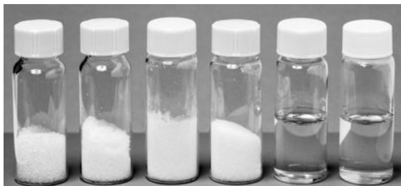
Figure 2.8. DESs components mixing stages which affords the liquid and homogenous eutectic.
