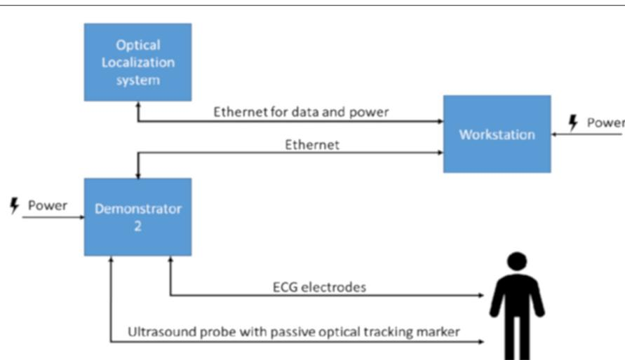
**FIGURE 2** | Scheme representing of the acquisition system flow.
