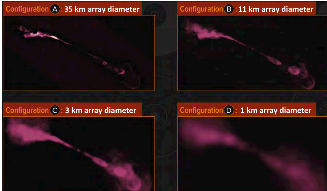
Figure 2.4: Radio source Hercules A shown in all four VLA configurations. The longest baseline of each configuration is given in kilometers. Images are adapted from NRAO/AUI/NSF.
