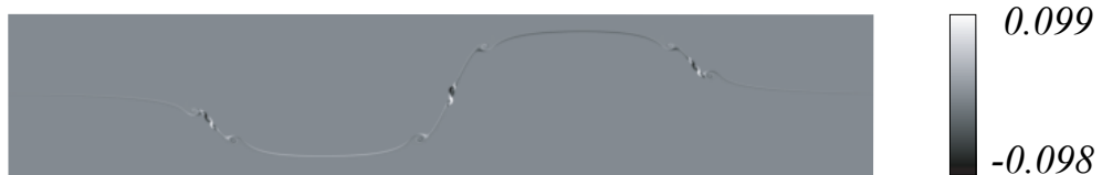
Figure 19: Convergence of numerical algorithm for the “hook with sliver” initial data. Plotted here is the density difference at t = 2.8 , generated by subtracting off the density from computations with 512 and 256 (vertical) nodes. Only the central portion (1/3 of the total length) of the channel is shown. For initial conditions that do not smooth the density jump, the resolution error becomes noticeable along the interface, where slight differences in its position in addition to numerical diffusion lead to nonzero density differences between the two computations.
