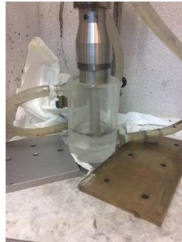
Figure 17 Example of ultrasonication instruments for laboratory dispersion of nanofillers.
