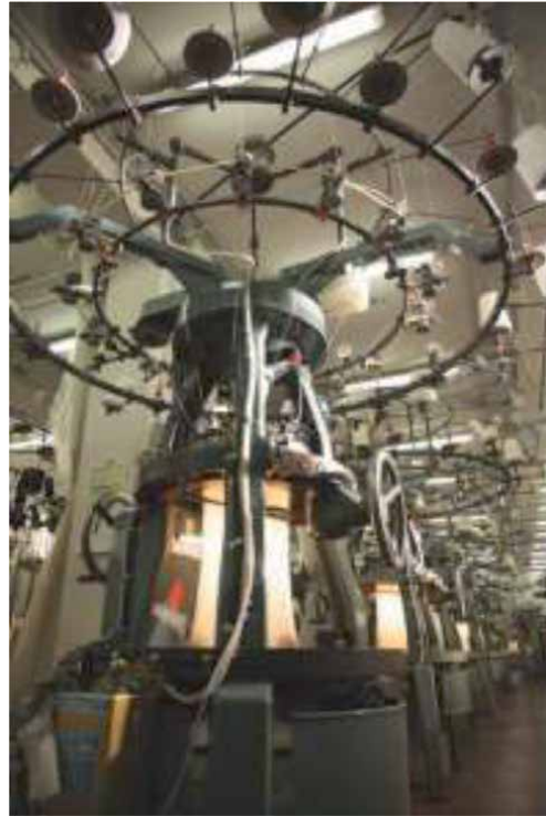
Figure 2. Tubular knitting machines. Source: Oscalito.
