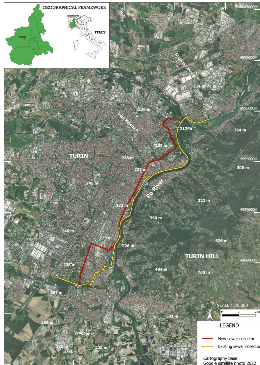
Figure 1. Location of the new sewer collector near the Po bed in the eastern sector of Turin.
