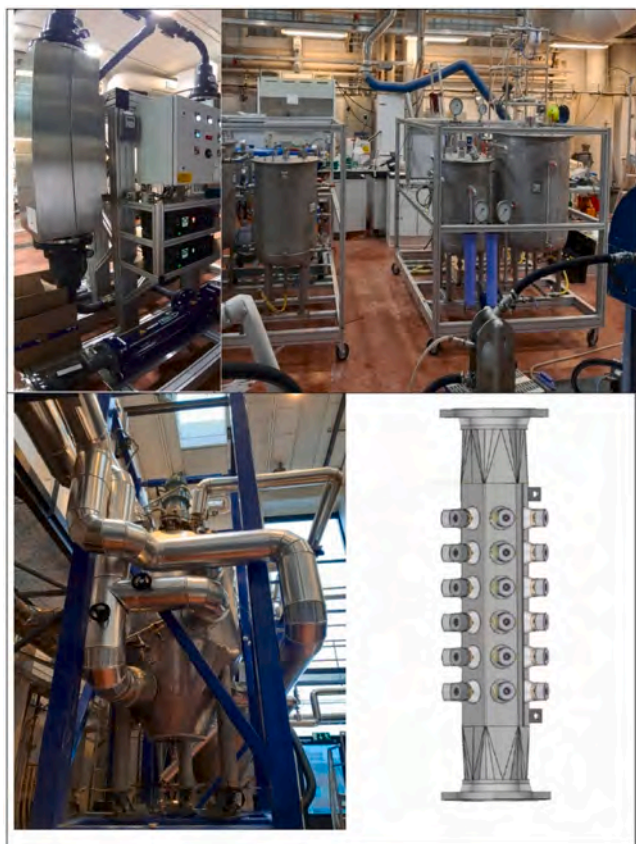
Fig. 5. Semi-industrial plant for US-assisted wheat-straw delignification. Reprinted with permission from Elsevier (Calcio Gaudino et al., 2022).
