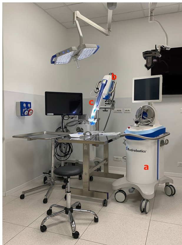
Fig. 1 Flex ® Robotic System consisting of two transportable main units and a flexible robotic endoscope: a Console, and Flex ® Drive, b Flex ® Cart and Base, c Flex ® Drive
