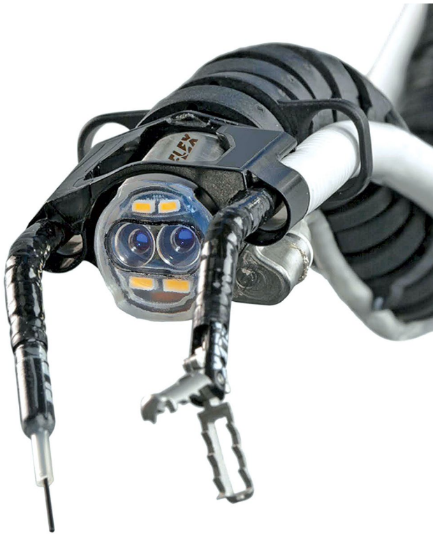
Fig. 2 The robot's flexible distal end including two working channels with a needle-knife and grasper
