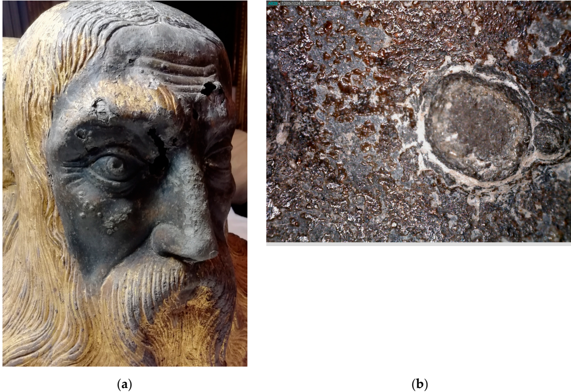
Figure 3. Globular alteration products: (a) photography of the face of Saint Venanzio; (b) details acquired by optical microscopy on the face of Saint Ruffino.
