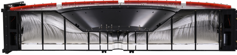
Figure 57. Photograph of one half of the FV0. The optical fibers connect the scintillators to the PMTs on the rim of the support structure, the black structure seen here. The center wall has been removed to show the scintillator, the surface matrix structure, and the optical fibers.
