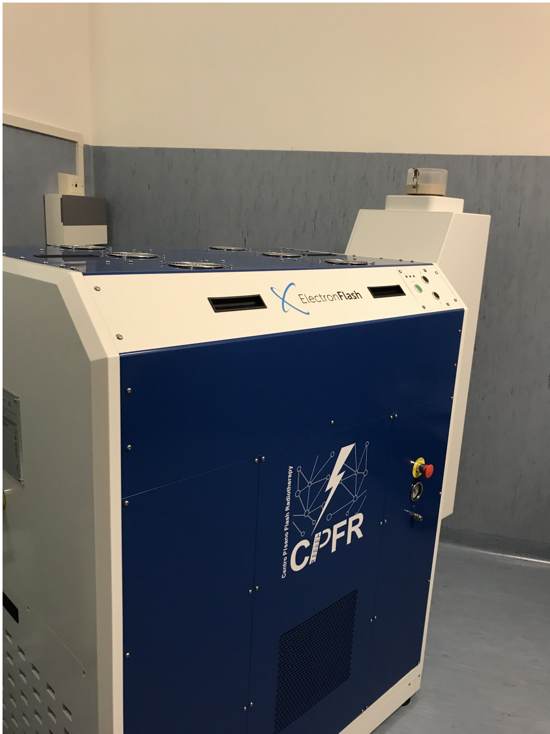
FIGURE 5.10: ElectronFlash accelerator of 7 MeV and 9 MeV located at the Centro Pisano Flash RadioTherapy (CPFR) in Pisa, Italy.
