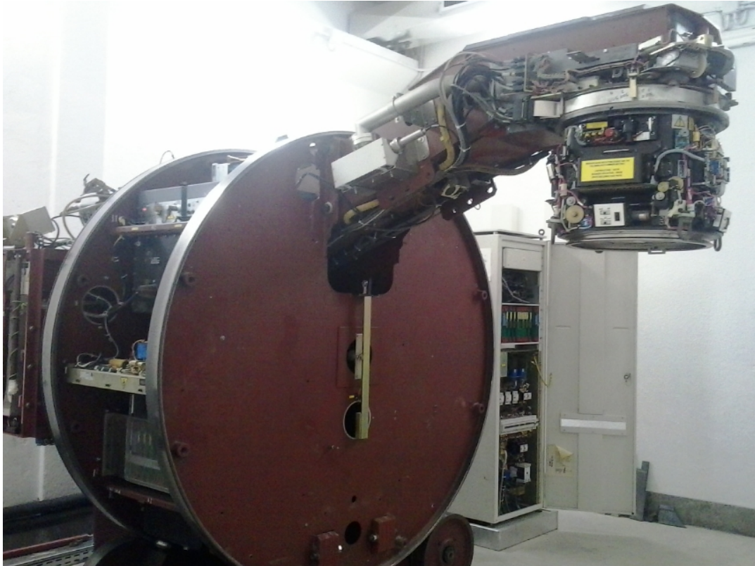
FIGURE 5.1: Linear Accelerator (Linac Elekta SL 25 MV), entirely dedicated to research, located at the physics department of the University of Turin (Italy).
