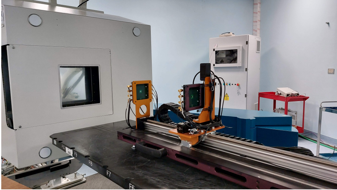
FIGURE 4.3: Picture of the experimental setup (2) used at CNAO to measure the time resolution for a single crossing. The system is based on a telescope configuration of two silicon sensor.
