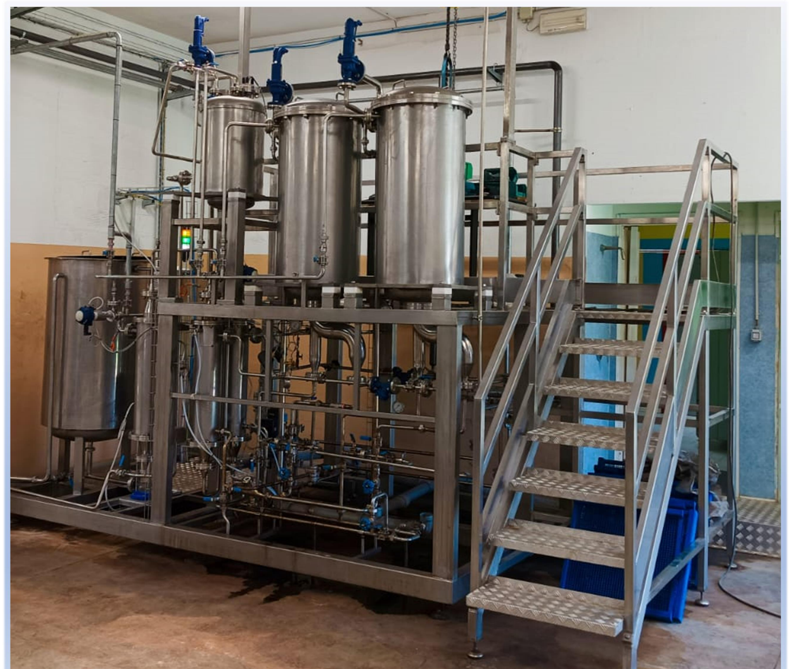
Semi-industrial plant for subcritical water extraction
