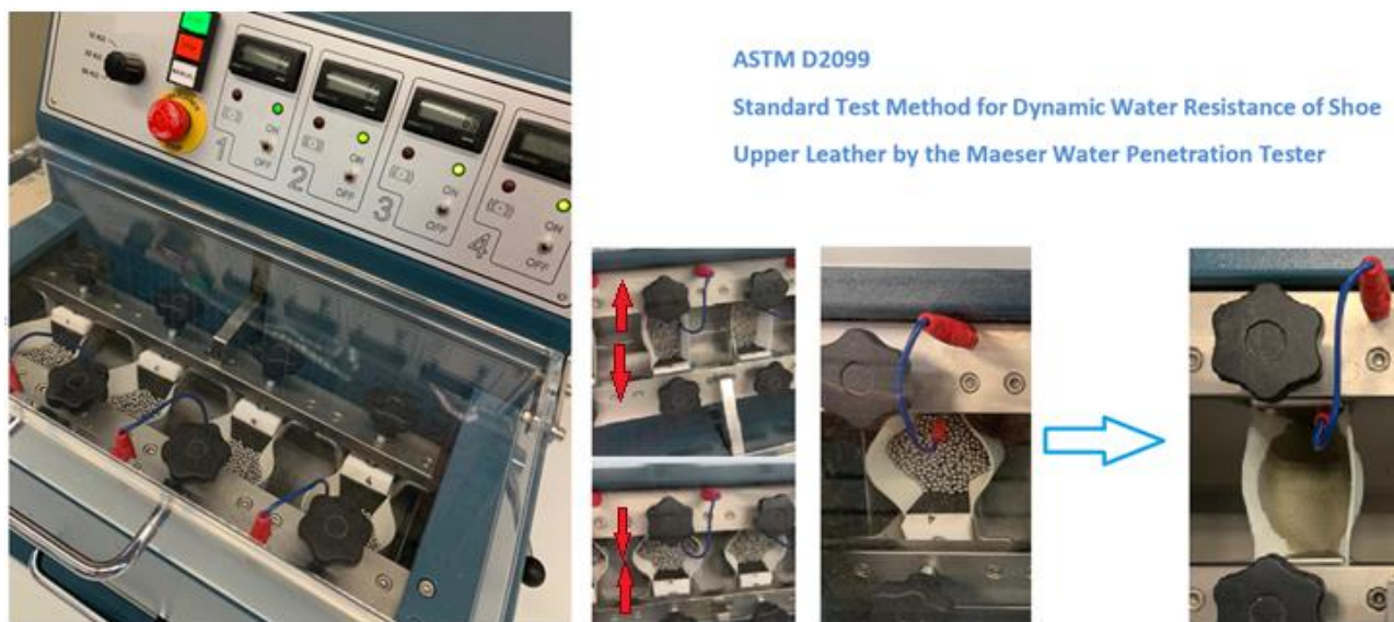
Figure 2.6.10. Maeser Water Penetration Tester. On the right the situation at the beginning and at the end of the test of a leather sample can be observed.
