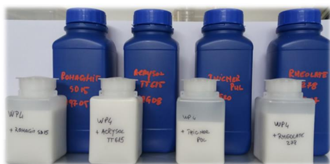
Figure 3.4.3. The selected thickening agents (ROHAGIT SD 15, ACRY SOL TT -615, THICKENER PUL, and RHEOLATE 278) added to the formulation.
