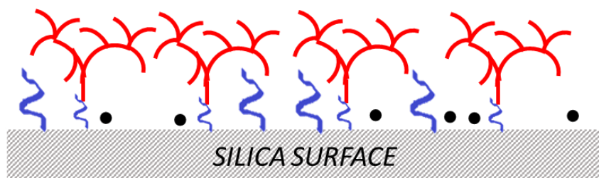
Figure 2.5.6. Schematic representation of the different moieties that can interact with water vapors: the blue one is representative of the APTS, the black dots of the non-reacted silanols, while the ISOST is represented by the red structures.
