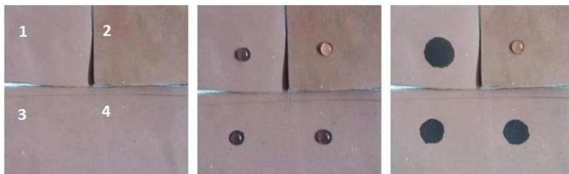
Figure 2.6.2 Deposition and water drop tests (t=0 sec in the center, t=32 sec on the right) on leather samples: 1) non-treated leather 2) leather treated with perfluorinated waterproofing agents, 3) leather treated with acrylic polymer and 4) leather treated with acrylic polymer + AluC-ISOST.
