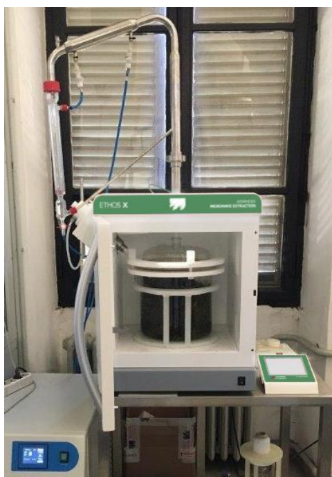
Figure 13. ETHOS X, MAHD set-up.
