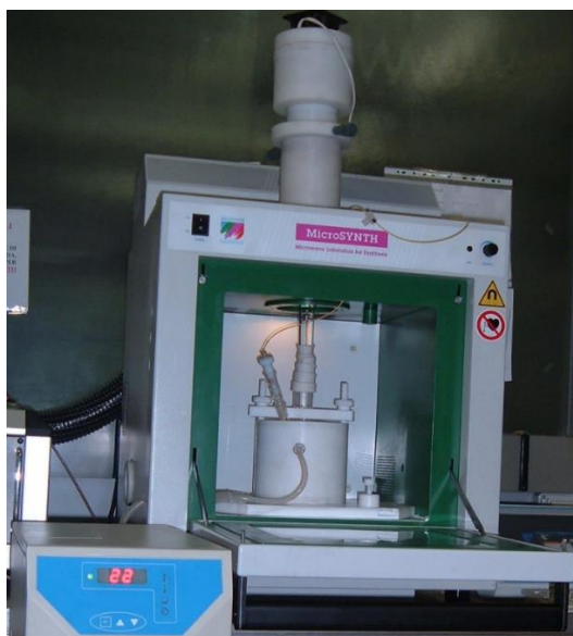
Figure 7. MicroSYNTH MW reactor combined with a Pyrex® horn.
