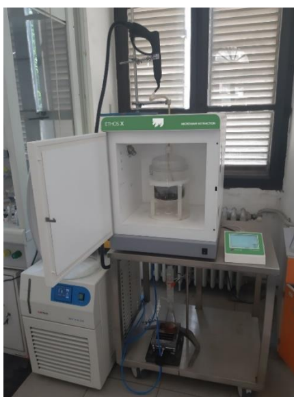
Figure 14. ETHOS X, MAHG set-up.
