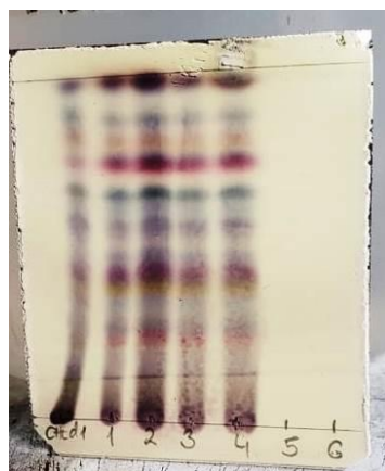
Figure 15. TLC of conventional extract and samples obtained in SCO 2 E by periodical sampling. First line represents conventional extract and the following lines show SCO 2 E samples.
