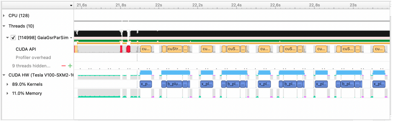
Figure 5: Output of the NVIDIA Nsight Systems profiler [14] for a run of the MPI+OpenACC code with 4 iterations of the LSQR algorithm. The code is parallelized on 4 MPI processes on one node of Marconi100, and thus on 4 GPUs, and the system occupies a memory of 10 GB. This output shows the portion of the OpenACC code from line 4 to line 17 of Figure 3.
