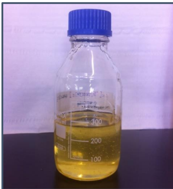
Figure 16. Picture of the yellow viscous liquid obtained in the Ti(IV) complex synthesis
