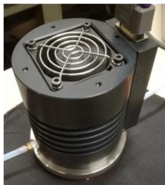
Figure 53. UP: Photoreactor scheme. BOTTOM: Photocatalytic reactor used for the gas-solid photocatalytic test (LEFT) (For a full description see Ref.2) and UV spectra emission centered at 365 nm of the photoreactor (right).
