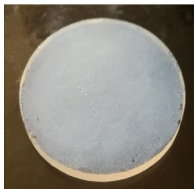
Figure 54. Example of the TiO 2 film used for the gas-solid photodegradation experiments.
