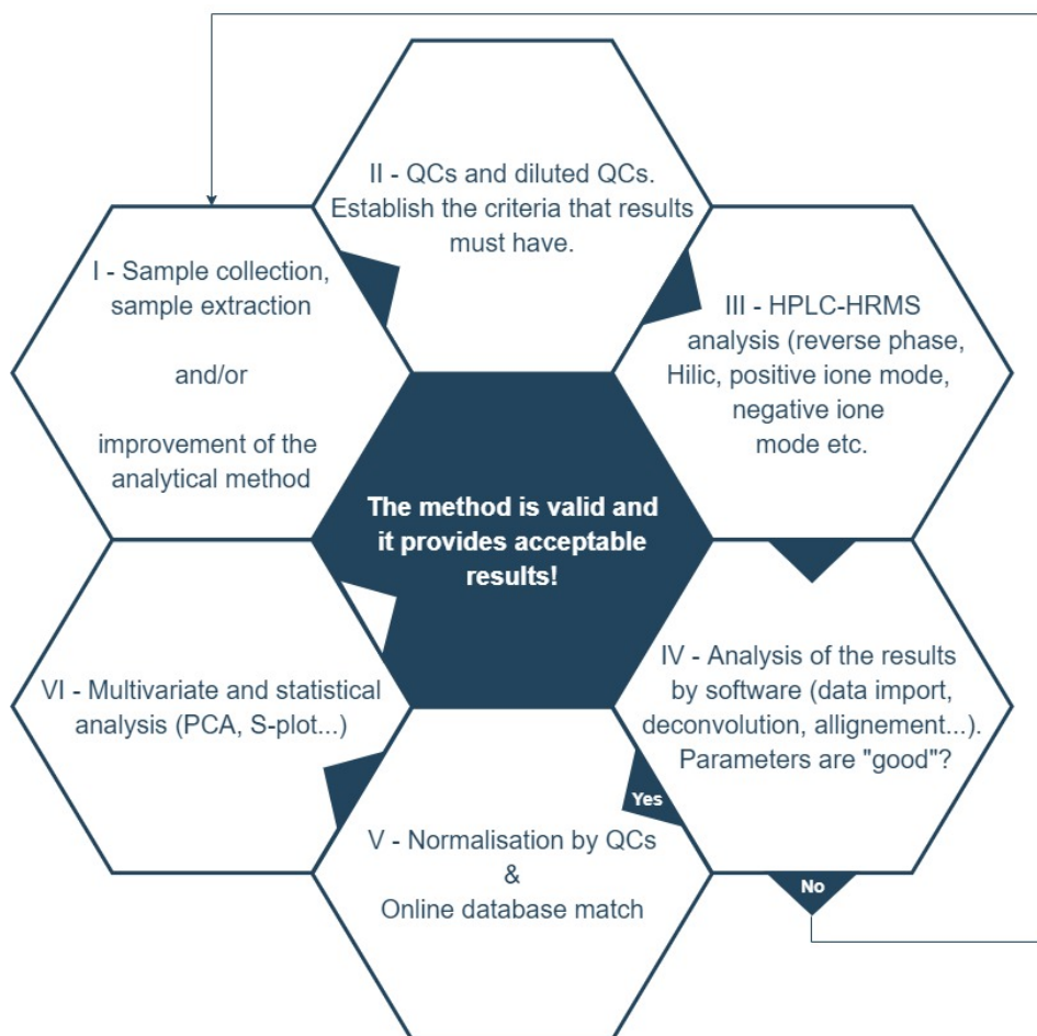
Figure 4.4.: Flowchart for global metabolomics LC-MS method apply in our Lab. The different steps will be deeply discussed in chapters 9 to 12
