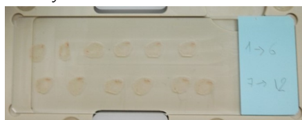
Figure 10.6.: Cryostat tissue sections by placed onto a glass ready for DESI-MS
