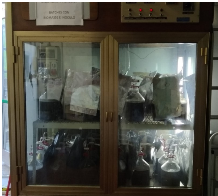
Figure 28: Batches ready for BMP trials inside the climatic chamber used to keep constant the process temperature at mesophilic conditions (40 °C ± 2 °C)
