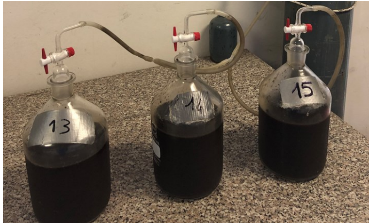
Figure 27: Batches prepared with mixture of inoculum, water and biomass and subjected to nitrogen flushing to provide the anaerobic conditions necessary to start AD process.
