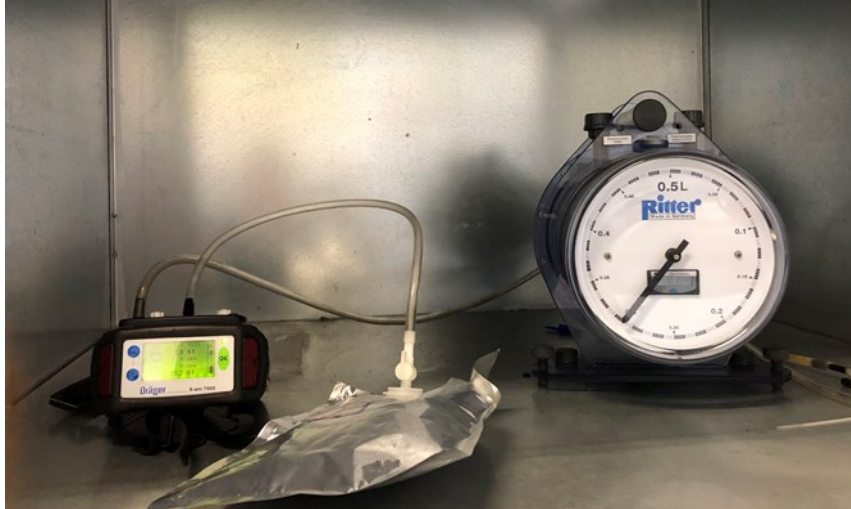
Figure 29: The equipment used to measure the volume and the chemical composition of biogas produced during the BMP tests.
