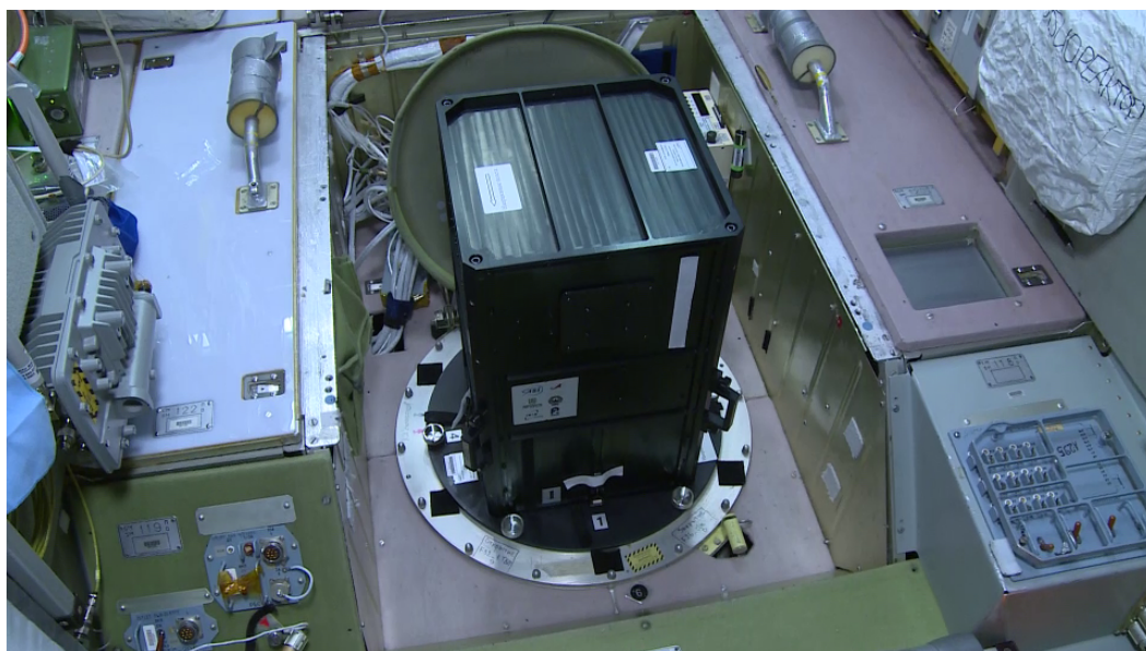
Fig. 3.12: Picture of the Mini-EUSO telescope installed for observations from the ISS, mounted on the UV transparent window of the Zvezda module. The velocity vector of the ISS is usually oriented towards the bottom of the picture, on the side marked as '1' (Bacholle et al., 2021).
