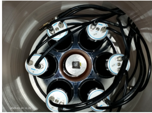
Fig. 5.9: The F2 specimen of Cavezzo just before the measurement, placed on the top of the GEM90 HPGe detector and surrounded by the NaI(Tl) annulus. The six photomultiplier tubes on the top of the NaI annulus are also visible (Bizzarri et al., 2023).
