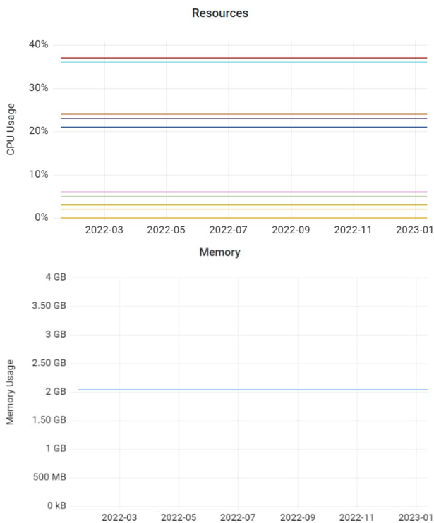
Fig. 6. Resource utilizations of VPC A and VPC B: CPU usage of all utilized cores in different colours (top graph) and memory usage of the VPC application (bottom graph).
