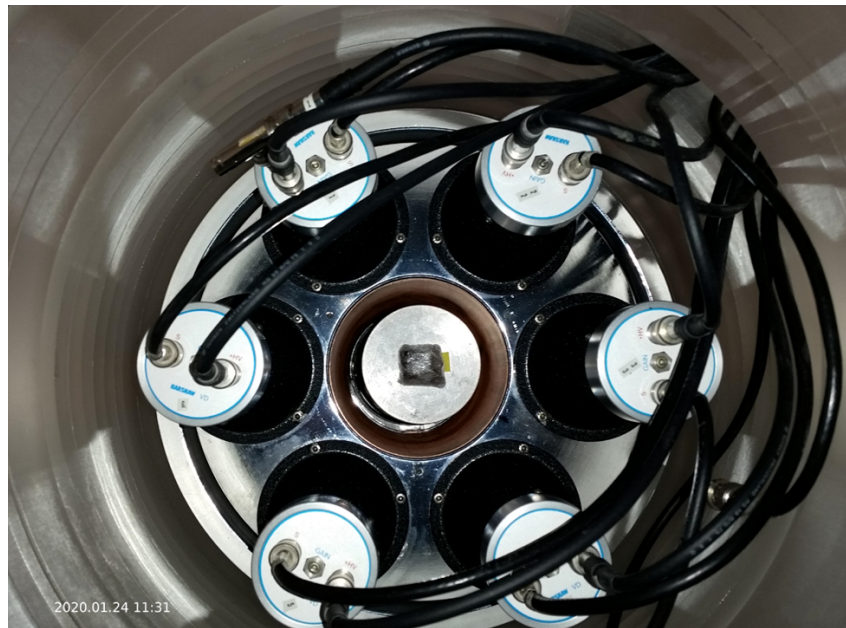
Figure 3.4: GEM90 HPGe detector surrounded by the NaI(Tl) annulus. The F2 specimen is placed on top of the germanium crystal. The six PMTs on the top of the NaI annulus are also visible.
