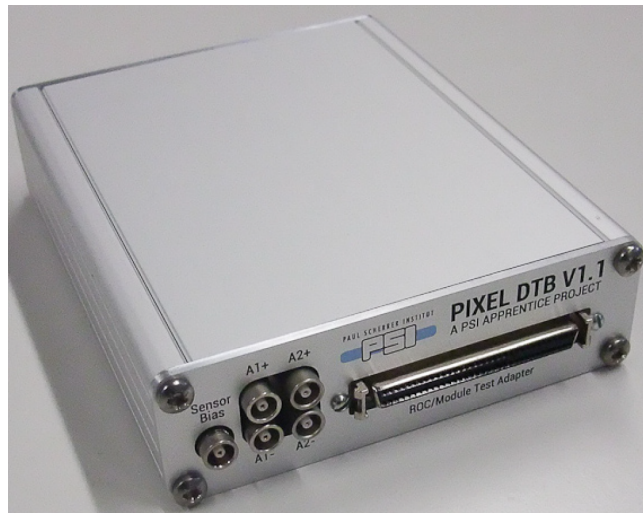
Figure 5.12: Picture of the Digital Test Board (DTB).
