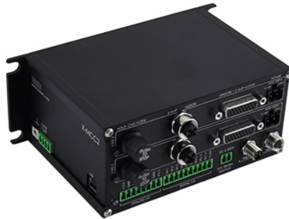
Figure 5.8: Picture of the X-MCC2 motor driver.
