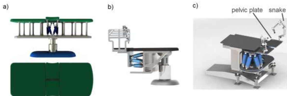
Figure 3 Different possibilities for hexapod position; c) solution has been chosen
