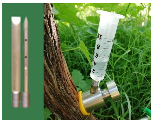
Fig. 2 – A representation of the lenticular shaped perforated blade on the left. On the right, the infusion treatment in progress.
