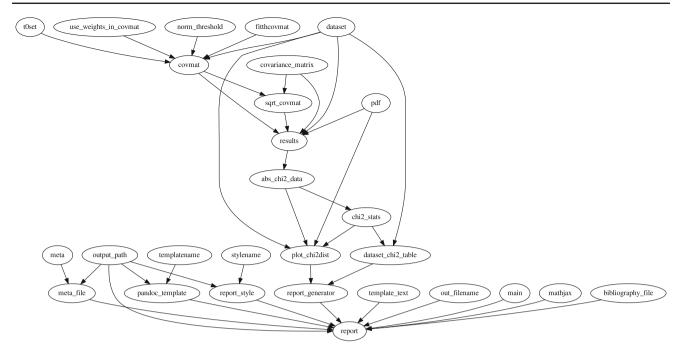
Fig. 2 Direct acyclic graph corresponding to the run card provided in Fig. 3. The graph shows the inputs extracted from the run card, such as pdf (the PDF set) and the dataset, the intermediate steps required for the  $\chi^2$  computation (such as evaluating the covariance\_matrix),
