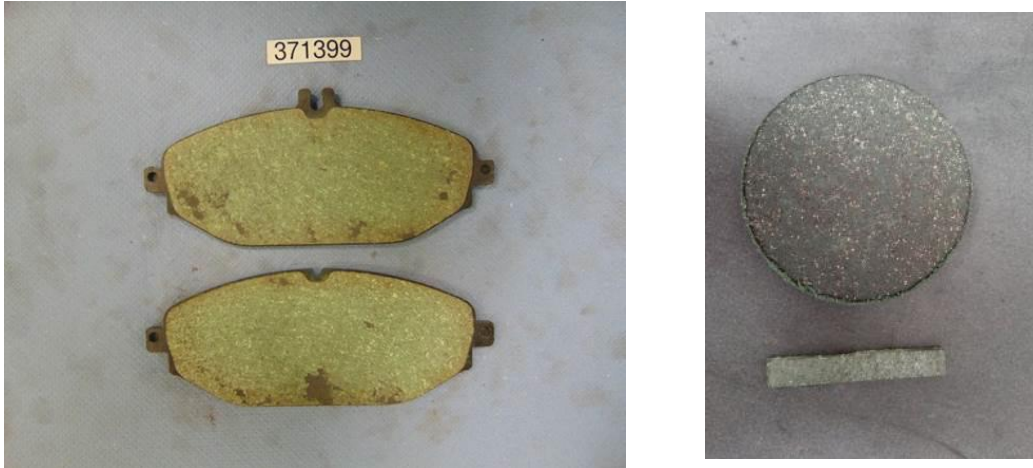
Figure 4.15: On the left, there is a grinding pad to 3 mm from the metal back plate, the figure shows the underlayer distribution. On the right, the circular underlayer mold ( d = 90 mm) and below this is the specimen for the analysis of DMTA.
