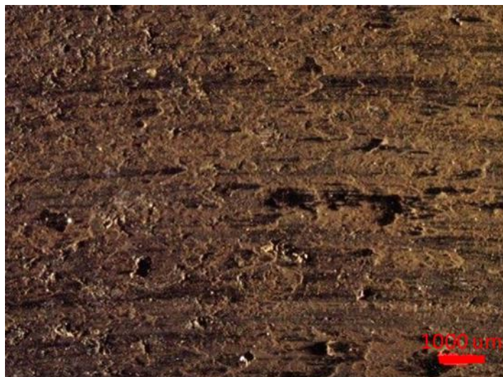
Figure 5.14: Optical image of the reference Low Steel material obtained with optical microscope. Lateral light, zoom 10X.
