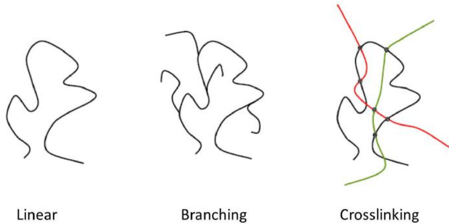
Figure 3.1: Polymer architecture, it strongly influences the characteristics of the material [21].
