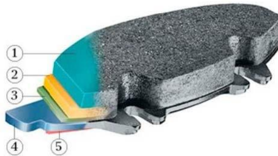
Figure 1.2: Composition of a generic brake pad [2].
