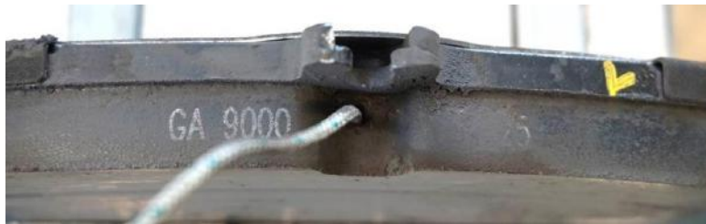
Figure 4.23: Thermocouple to measure the temperature of the underlayer. It is fixed at 3 mm above the metal back plate.
