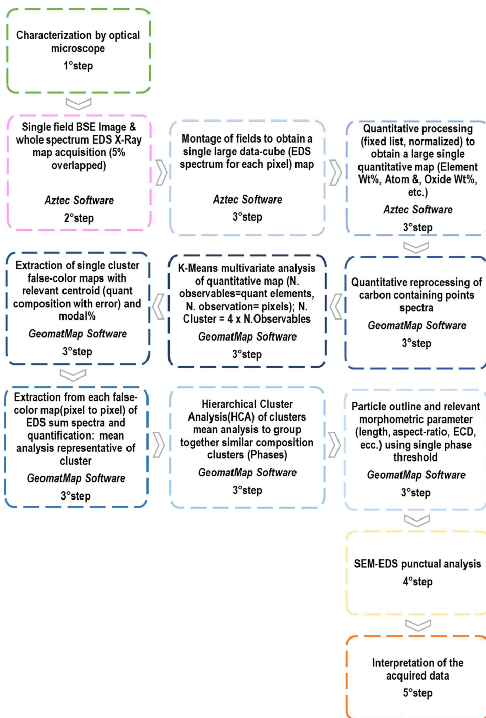
Figure 5.24: Flow chart of analytical protocol for the petrographic study of mortars.
