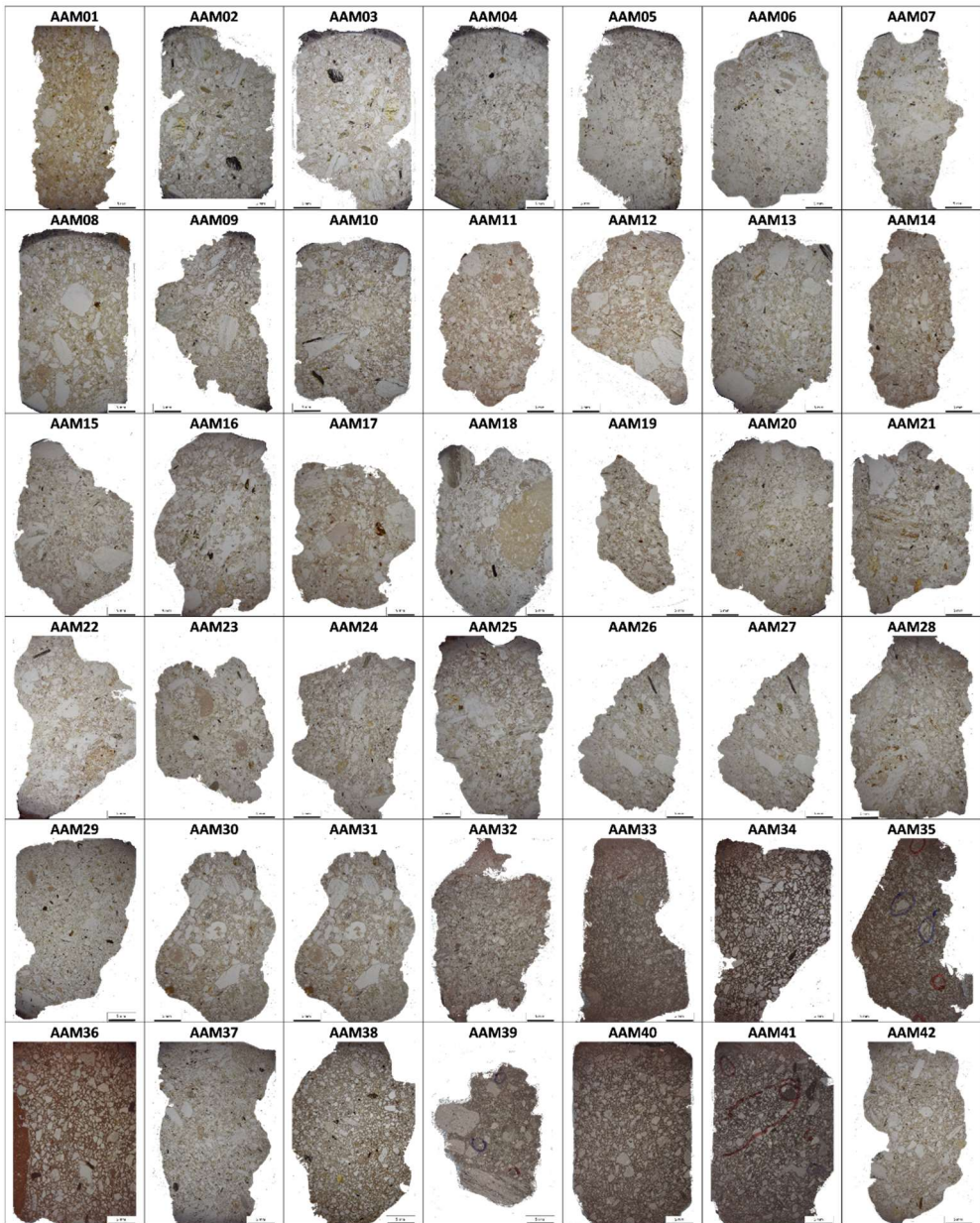
Figure 5.12: Thin section of the samples of Roman Theatre of Aosta, Optical Microscope, // pol.
