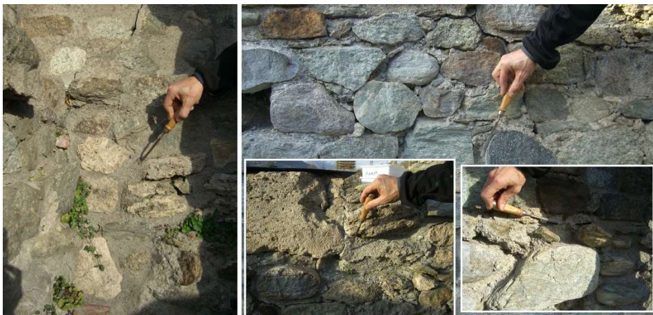
Figure 5.9: Sampling of centimeter-sized mortars specimen performed by a chisel.
