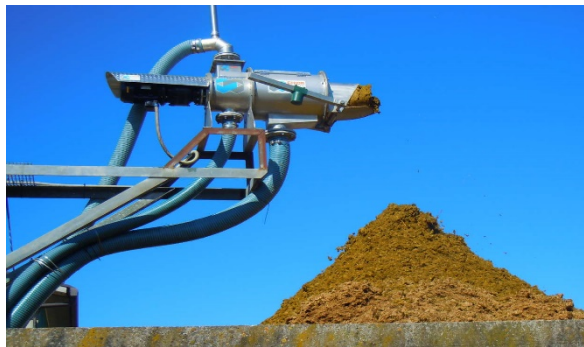
Figure 4: Mechanical digestate separator; the digestate enters the upper tube, the liquid part exits in the tubes below and the solid fraction laterally.
