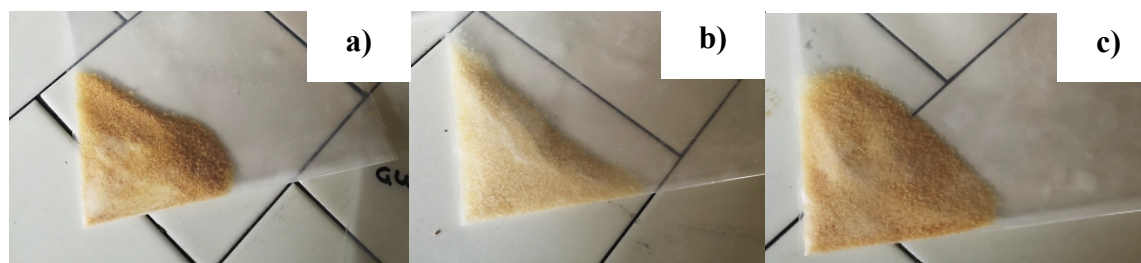
Figure 93: a) Sodium alginate based nanosponge; b) carrageenan-K and c) 1,4-butylsulton based nanosponge (post synthesis).
