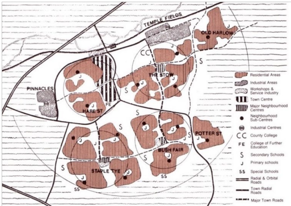
1: Diagrammatic Masterplan of Harlow in which we can see the separation between a) Radial & Orbital Roads, b) Town Radial Roads and c) Major Town Roads. Source: Sir Frederick Gibberd, The design of Harlow (Harlow: Information Services Dept., Harlow Council in association with Harlow Development Corporation, 1980).
