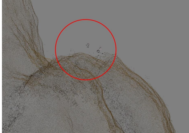
Fig. 3.20. The noisy points the dense point cloud that are to be cleaned
