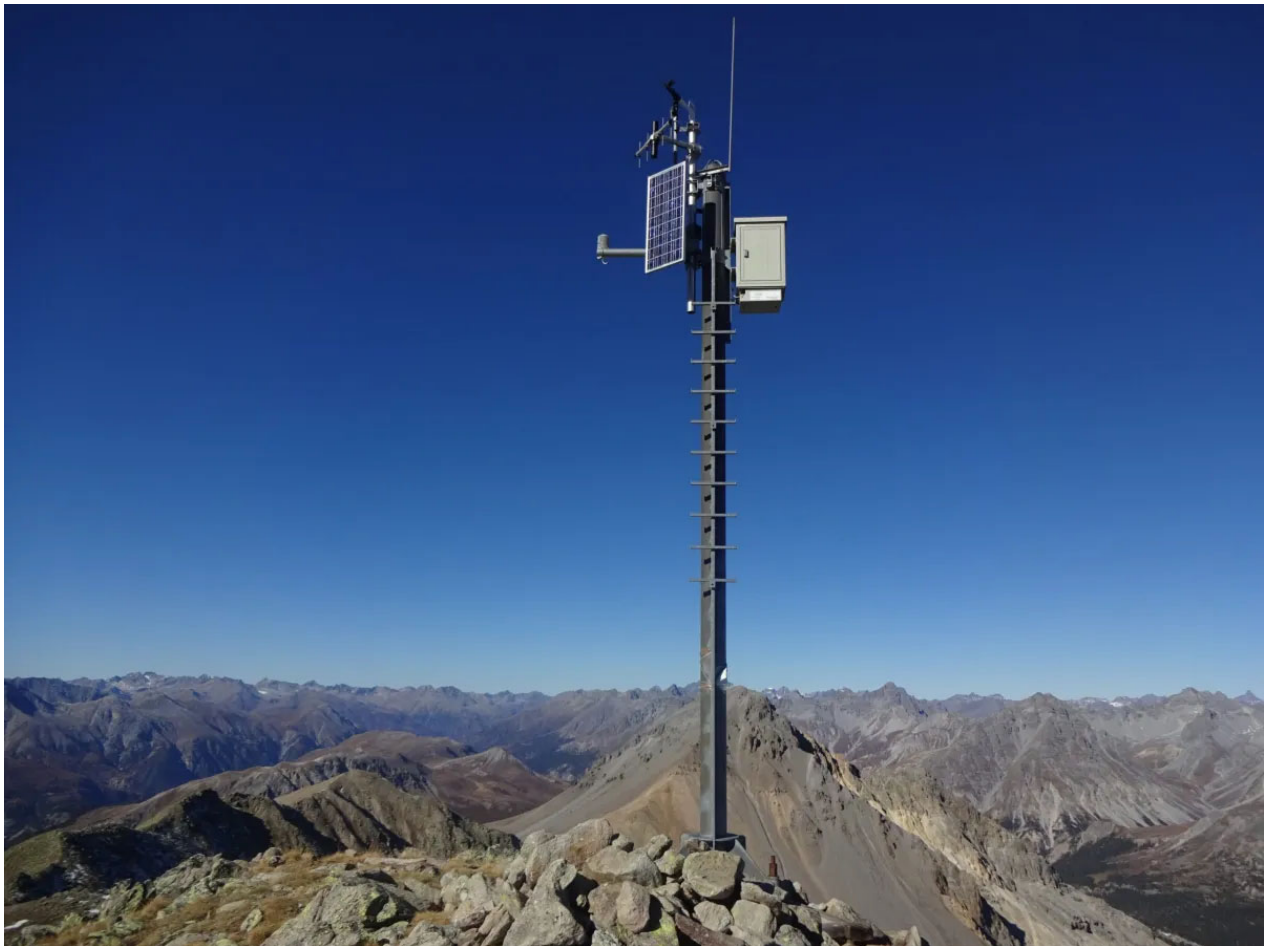
Automated weather and snow cover station on Piz Dora (2,951 meters above sea level) in the Engadine Alps, Switzerland (photo taken in October 2021). Mountain weather stations such as this one are relatively few, due to difficult challenges in operation in such an extreme environment. Credit: Sven Kotlarski (MeteoSwiss)
