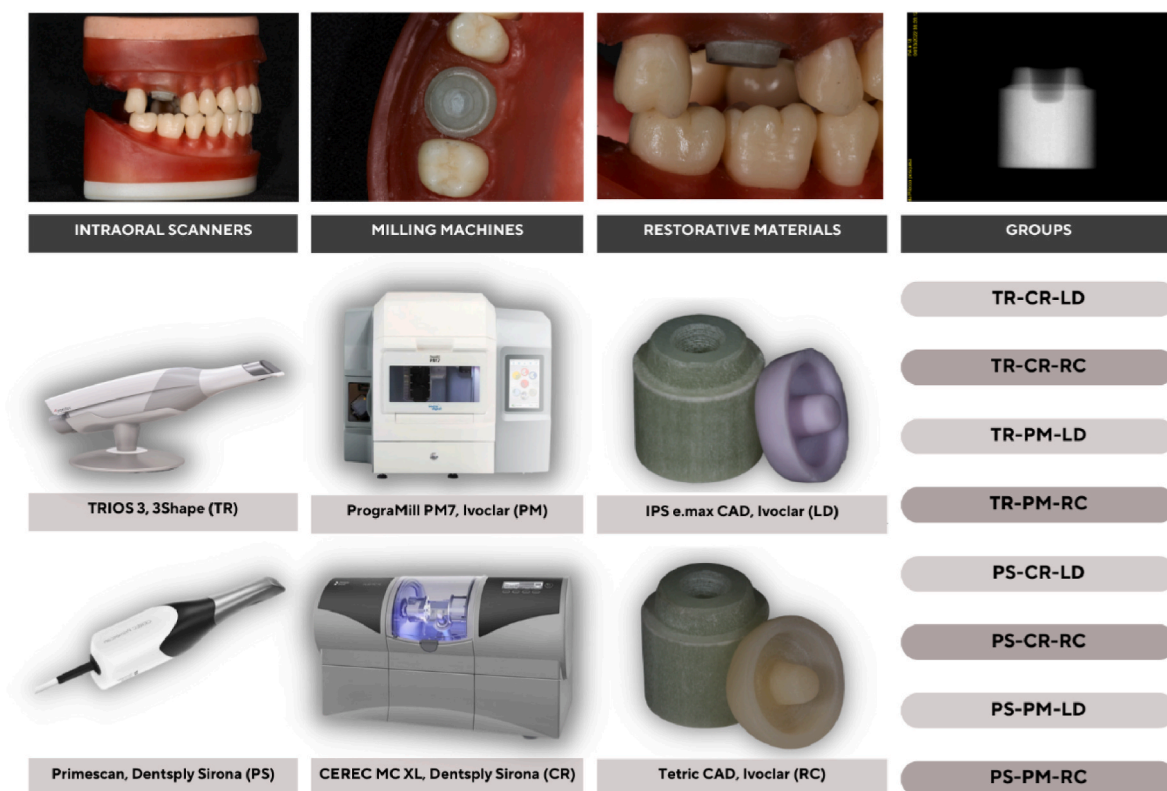
Fig. 1. Flow chart of the study design and illustration of the adapted typodont model for the endocrown scanning procedure (TR, TRIOS 3; PS, Primescan; CR, CEREC MC XL; PM, PrograMill PM7; LD, lithium disilicate; RC, resin composite; n = 10).
